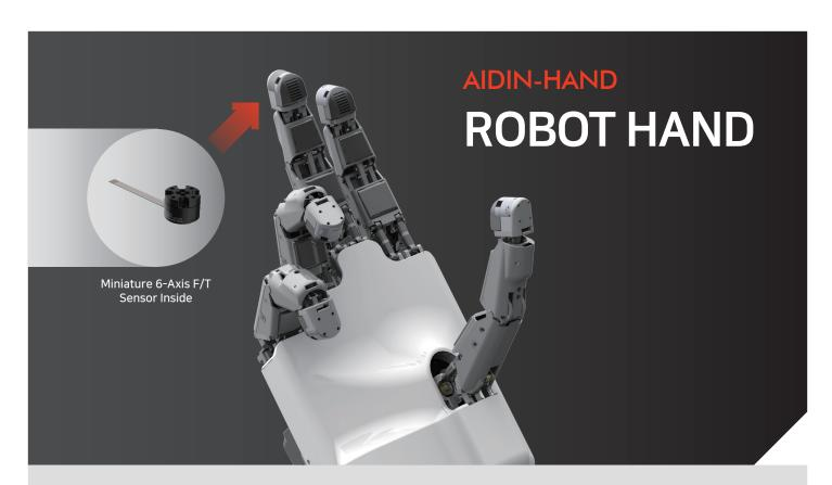
AIDIN ROBOTICS' self-developed robot hand is equipped with Miniature 6-axis F/T sensors (AFT20/50) at each fingertip. This enables precise and delicate grasping operations that are difficult to achieve with conventional grippers, supporting more refined and versatile object handling.
